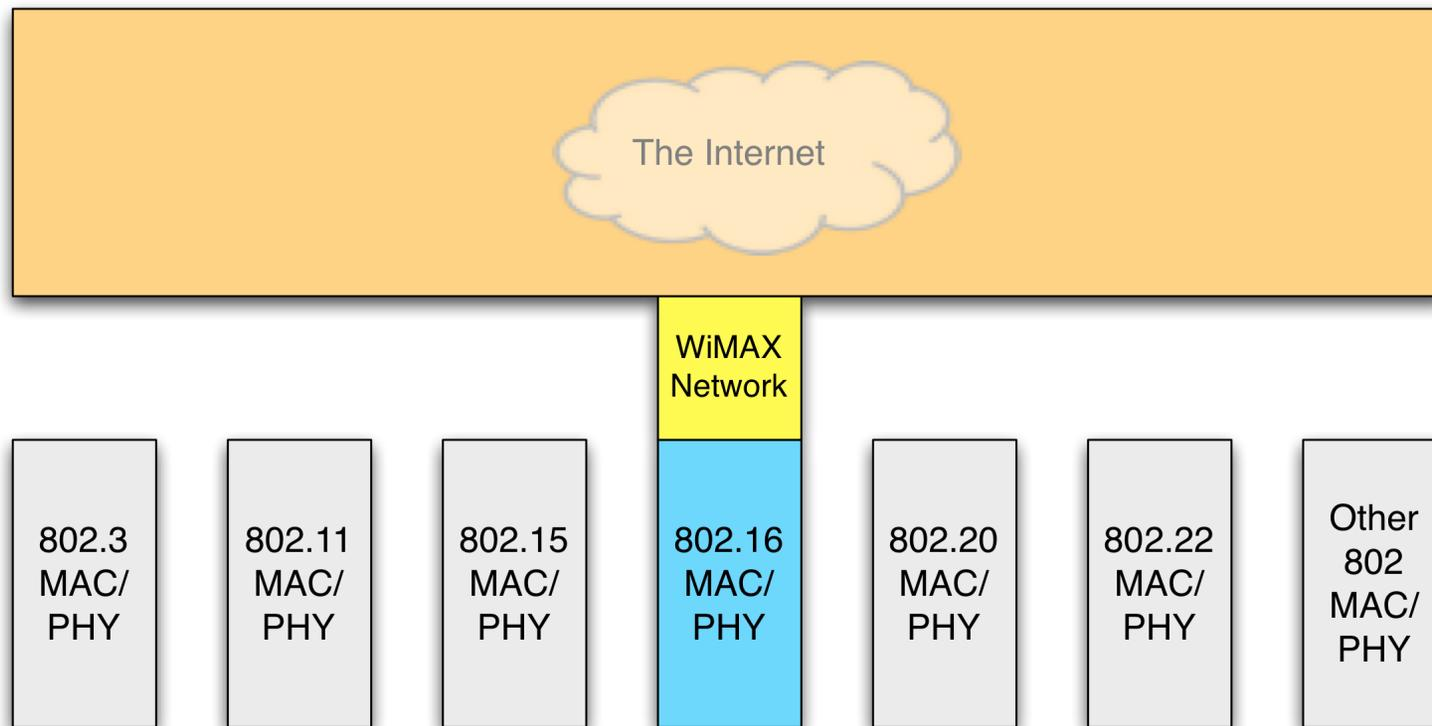
WiMAX Network provides operator-required services to 802.16 devices: authentication, provisioning, mobility management, QoS management, roaming...
